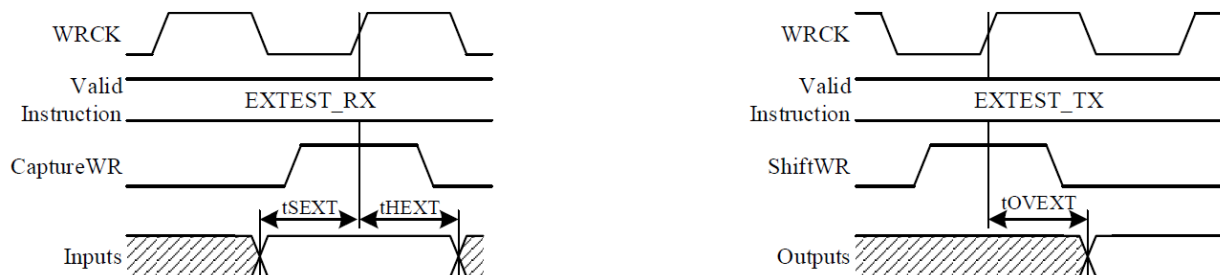
Figure 107 — IEEE1500 EXTEST_RX and EXTEST_TX Instruction Related Timings
